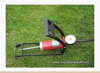
Even so, we wouldn't really describe this as an air compressor, because its job is really to move air from the atmosphere into tires. A compressor is normally designed to **make use of compressed air** in some way, for example, by powering a jackhammer (pneumatic air drill).
